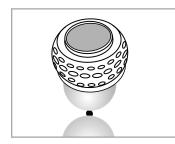
5: Smooth side of magnet should be showing. Place clasp so that magnet is *straight up* while glue is drying. Laying it down could cause the magnet to slip and prevent the clasp from closing properly.
