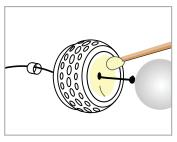
2: Apply a thin layer of epoxy on the smooth cupped area. Then pull to glue pearl into clasp. Pearl knot should pull into the hole.
