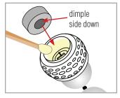
4: Use an emery board or nail file to lightly rough up the sides and dimpled side of the magnet. Apply epoxy over crimp and sides of clasp. Place magnet DIMPLE SIDE DOWN in clasp. Firmly press the magnet and wipe off any excess glue that seeps out. Use a cloth or Q-tip dampened with rubbing alcohol.
